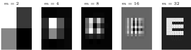
Fig. 3. Resolution-limited reconstruction of a 32 \times 32 image, from its moments up to order (m, m) , using Lemma 2 and Haar coefficients.
