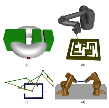
**Fig. 5** The four benchmarks used to test the AtlasRRT planner. (a) A point moving on a torus with obstacles and a narrow corridor. (b) The Barret arm solving a maze problem. (c) A planar parallel manipulator moving a peg out of a cul-de-sac. (d) Two Stäubli Rx60 industrial arms collaborating to move a cylindrical bar.
