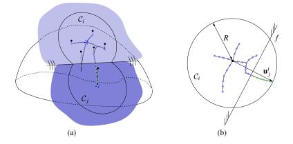
**Fig. 3** (a) When a RRT leaves the validity area of chart  $C_i$ , a new chart,  $C_j$ , is created and their respective sampling areas are coordinated so that they do not overlap. (b)  $C_j$  adds an inequality, f, to  $C_i$  reducing its actual validity area. Note that after adding f, the nodes in green move from  $C_i$  to  $C_j$ .
