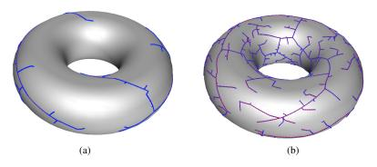
**Fig. 1** Two RRTs built on a torus-like manifold after throwing 500 samples. (a) With an ambient space sampling, the exploration is focused on the exterior regions of the torus and many samples do not produce any tree extension. (b) With an AtlasRRT, the diffusion process is largely independent of the ambient space which improves the coverage.
