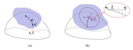
Fig. 2 (a) A chart  $C_i$  is implemented as a mapping  $\mathbf{x}_j = \psi_i(\mathbf{u}_j^i)$  between the tangent space at  $\mathbf{x}_i$  and the manifold. (b) Growing a RRT on the manifold from a single chart. Black dots are the samples thrown in the tangent space and blue dots are points on the manifold forming the RRT branches. The inset shows the process of generating a branch by linear interpolation in the tangent space with steps of size  $\delta$  and successive projection.
