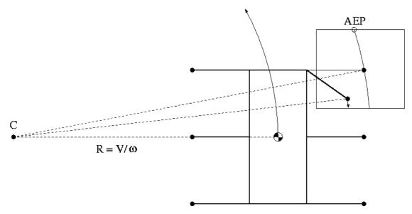
Figure 2. Target foot position for a leg near to reach its workspace limit.
