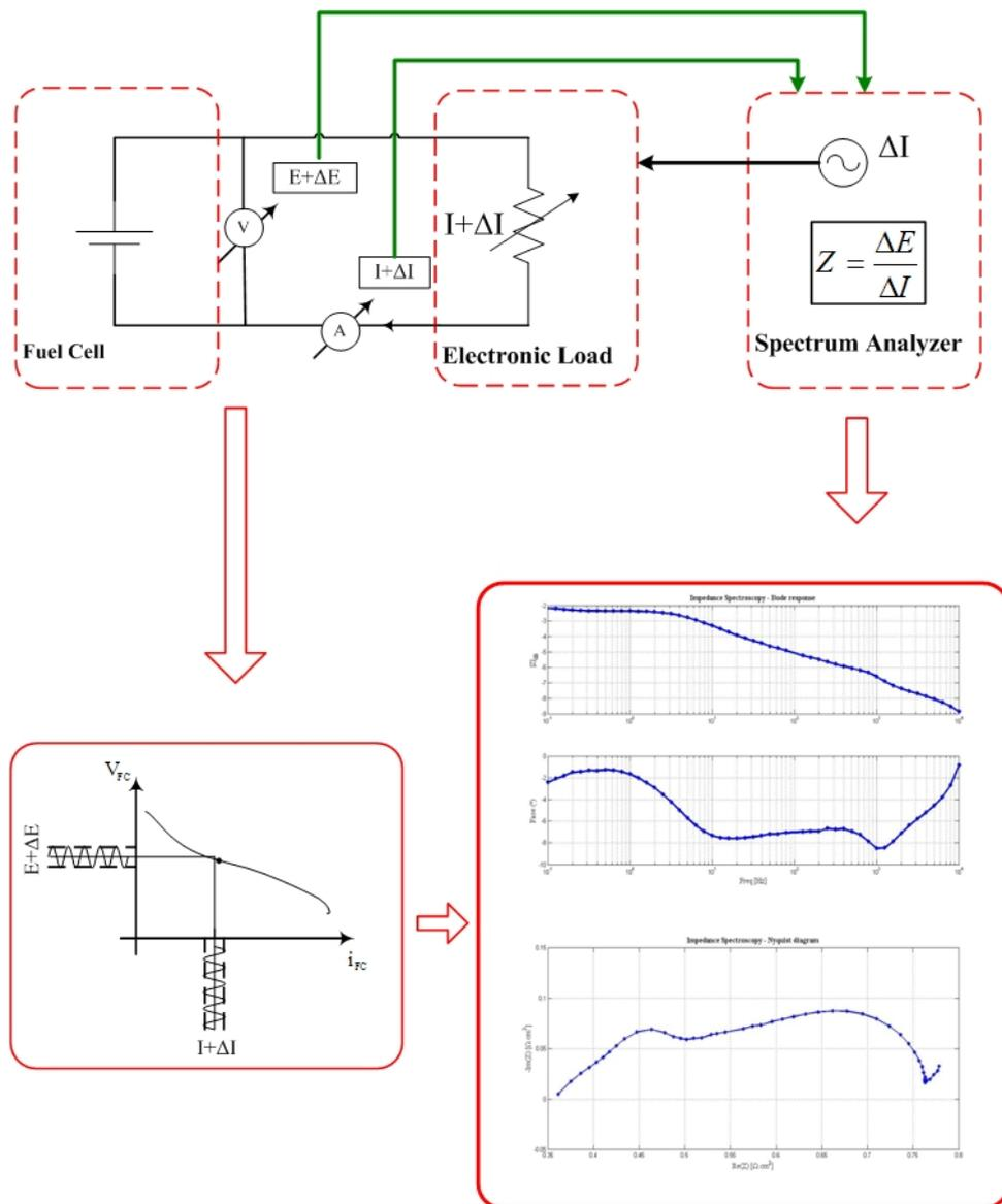
Figure 1 – EIS implementation and frequency response
