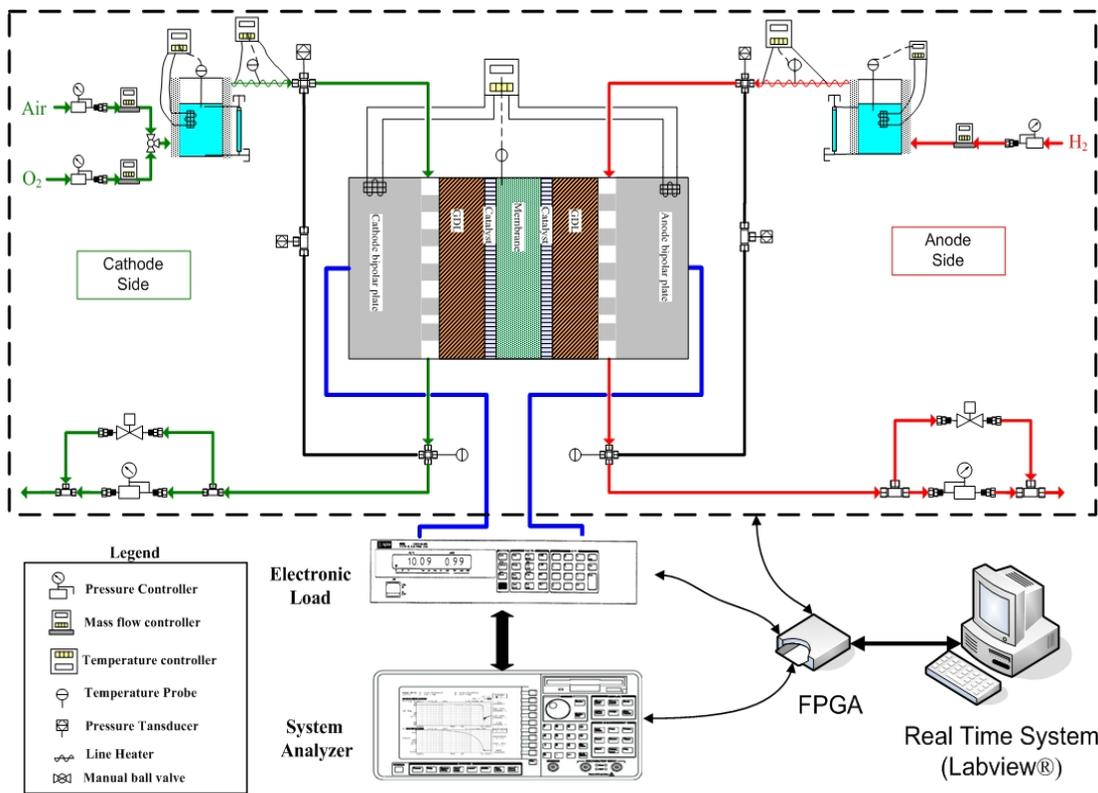
Figure 3 – Experimental setup description
