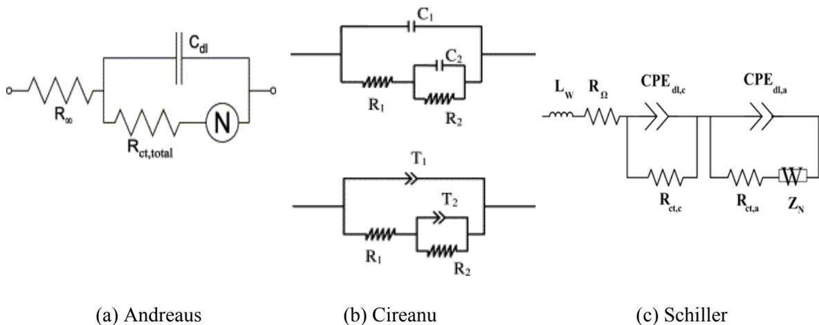
Figure 2 – Equivalent Circuit models
