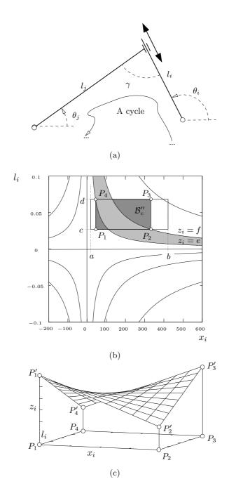
Figure 9: Dealing with slider joints. (a) A slider joint between links i and j. (b) Adjusting a box to fit a hyperbolic paraboloid  $z_i = x_i l_i$ . (c) The tetrahedron defined by the  $P'_i$ 's is a convex bound of this surface inside  $\mathcal{B}''_c$ .
