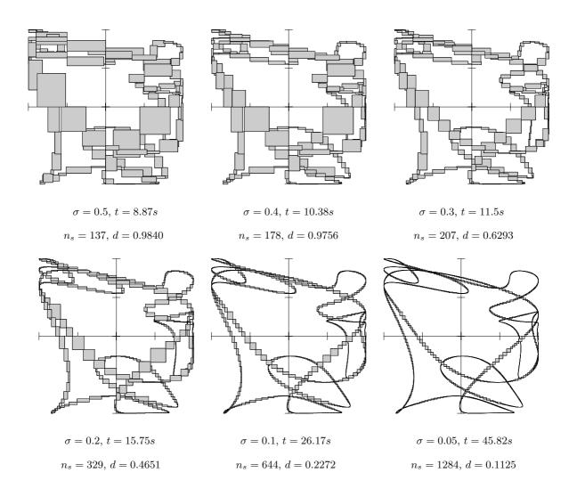
Figure 4: Output boxes at increasing resolution. The horizontal and vertical axes respectively correspond to  $\cos(\theta_2)$  and  $\cos(\theta_4)$ , spanning the range [-1,1] in all cases, with marks separated 0.5 units apart.
