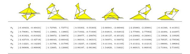
Figure 3: The six real solutions of the double butterfly linkage for  $\theta_6 = 1.175$  rad (67.38°), given in radians.
