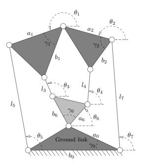
Figure 1: The double butterfly linkage.
