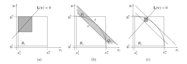
Figure 2: (a) Shrinking  $\mathcal{B}_c$  to fit the linear variety  $\mathbf{L}(\mathbf{v}) = 0$ . (b) Half-planes approximating the circular arc inside  $\mathcal{B}_c$ . (c) Smallest box enclosing the intersection of  $\mathbf{L}(\mathbf{v}) = 0$  with the half-planes in (b).
