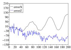
Fig. 10. Difference in millimeters between translation estimates provided by the laser and the vision subsystems for each frame.
