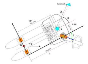
Fig. 1. Different reference frames defined in the forklift mobile vehicle.
