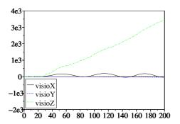
Fig. 7. Translati on im millimeters computed by the vision subsystem for each frame.
