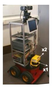
Fig. 1. The model for this nonlinear vehicle is used in the simulations, and is given in Appendix A. The Cartesian coordinates of the control point (x, y) are located on the projection center of the laser range scanner, and were porpousedly chosen not coincident with the vehicle axle center.
