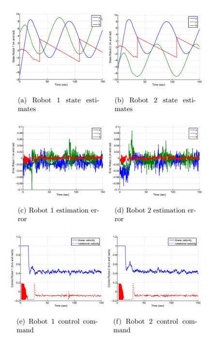
Fig. 3. State Estimation and Control using Feedback Linearization.
