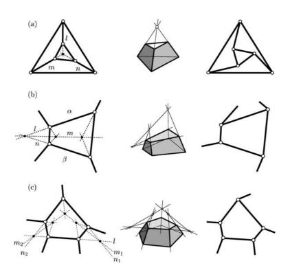
*Figure 4.* To be correct, the drawings on the left must verify the indicated concurrence conditions, since they hold on any of their spatial interpretations (center). These conditions allow to classify the drawings on the right as incorrect. The incidence structure implicitly considered in each example is that of its corresponding spatial reconstruction shown in the center.
