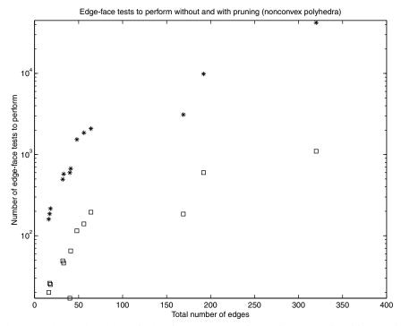
Fig. 18. Comparison between the total number of edge-face tests to perform without applicability pruning, that is, algorithm A (\*), and with a previous pruning step, that is, algorithm C ( $\Box$ ), in settings that include only nonconvex polyhedra.
