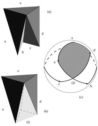
Fig. 6. (a) A pseudoconvex vertex, (b) its local convex hull, and (c) the corresponding convex subregion.
