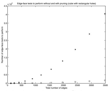
Fig. 21. Number of edge-face intersection tests to perform by algorithm C ( $\Box$ ) against the total number of edge-face pairings (\*) for the setting in which two cubes have an increasing number of holes.
