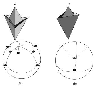
Fig. 13. The nodes and arcs (shown with dashed lines) of the region that represents v are disconnected from the remaining part of the spherical face orientation graph if the nonconvex arcs are eliminated. The nodes that correspond to faces of the polyhedron are shown as small ellipses. (a) Front view, (b) rear view.
