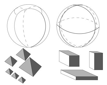
Fig. 7. Different polyhedra will have the same representation on the spherical face orientation graph if the relative orientations of the faces and adjacency relationships are preserved.
