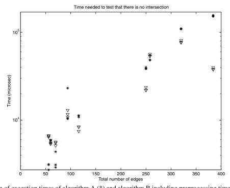
Fig. 17. Comparison of execution times of algorithm A (\*) and algorithm B including preprocessing time ( $\nabla$ ). Note that with preprocessing added, B outperforms A even for low complexities. The different results for each pair of polyhedra correspond to different relative orientations.
