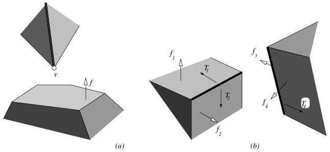
Fig. 2. (a) Applicable vertex-face contact, (b) applicable edge-edge contact.
