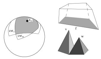
Fig. 12. For nonconvex polyhedra, situations may exist in which the same face is simultaneously applicable to several vertices: the corresponding node is contained in the common area of the overlapping convex subregions of these vertices.
