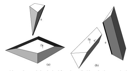
Fig. 3. (a) The candidate pairing e-f can only be obtained from the applicable v-f pair as no edge in the boundary of f can contact the edges stemming from the vertex, (b) the candidate e-f can only come from the applicable e-e' pair as no endpoint of either edge can contact the faces adjacent to the other edge.
