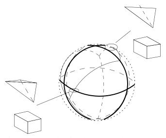
Fig. 11. Two examples of applicable contact between edges. The corresponding arcs intersect.
