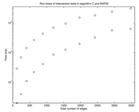
Fig. 22. Comparison of the execution times of the interference detection phase in algorithm C ( $\Box$ ) and RAPID ( $\circ$ ).
