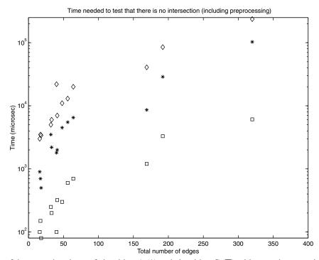
Fig. 19. Comparison of the execution times of algorithm A (\*) and algorithm C ( $\Box$ ) with a previous pruning step ( $\diamond$ ) in settings that include only nonconvex polyhedra.
