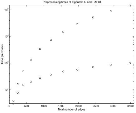
Fig. 23. Comparison of preprocessing times of algorithm C ( $\Box$ ) and RAPID ( $\circ$ ). Preprocessing is various orders of magnitude slower for the former. However, it has to be performed only once in settings where objects are only allowed to translate.
