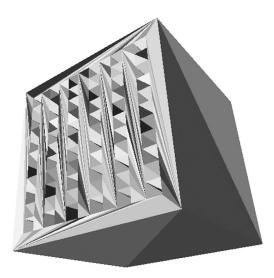
Fig. 20. The type of workpiece used to compare the performances of algorithm C and RAPID. The faces of the polyhedron (displayed here for the case of  $6 \times 6$  holes) were triangulated with an implementation of Seidel's algorithm (the code was obtained at http://www.cs.unc.edu/~dm/CODE/GEM/chapter.html). Remember that triangulation is a necessary previous step for RAPID but not for our algorithm.
