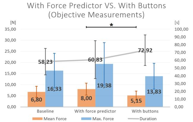
Fig. 2. **Three main objective measures considered.** Mean force exerted in orange, maximum force exerted in blue and duration in gray for the three experiments. Left axis in Newtons associated to both forces and right axis in seconds associated to duration. Statistical significance marked with \*:  $p < 0.05$
