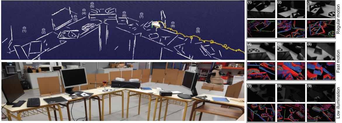
Fig. 6. Sequence: *Office\_large* using lines and events with DAVIS346. Fast motion and challenging lighting conditions are included in this sequence.
