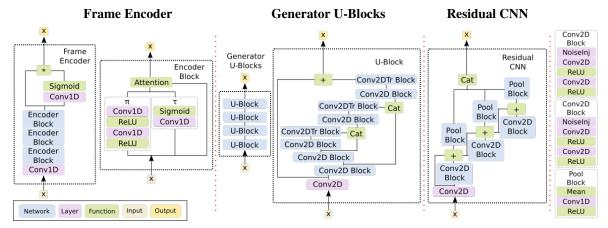
Figure 4. **Details of the architecture.** From left to right: Frame Encoder; Generator U-Blocks; Residual CNN. In each case we plot the general view of the block (left) and the fine detail of the structural elements (right). The Attention function is defined as:  $att(x, \pi, \tau) = \pi \tau + x(1-\tau)$ . The Conv2DTr denotes Convolution 2D Transpose, also called deconvolution.
