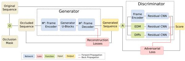
Figure 2. Overview of our architecture. An input masked sequence of 3D joint coordinates is fed into a fully convolutional and time preserving generator. The output sequence is controlled by a number of geometric constraints, including losses applied to the generator output and adversarial losses of three independent discriminators.
