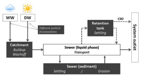
Figure 1 New Strucure of Quality Module SWMM-TSS
