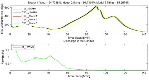
Figure 5 Flow rate and TSS behaviour out of Sewer 1
