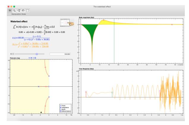
Figure 5. Waterbed analysis Interactive Tool: main screen (Costa-Castelló and Dormido, 2015).
