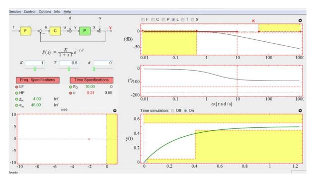
Figure 4. The Linear Control System Design (LCSD) (Diaz et al., 2017) main screen.
