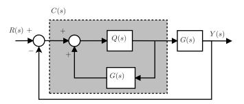
Figure 9. Closed-loop control system using affine parametrization.
