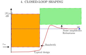
Figure 6. Sensitivity transfer function, S(s), specifications in the magnitude bode diagram.
