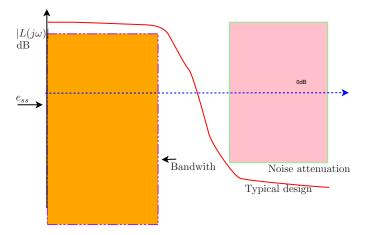
Figure 2. Open-loop transfer function, L(s), specifications in the magnitude bode diagram.
