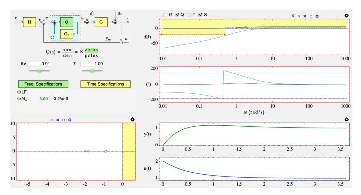
Figure 8. Closed-loop Interactive loop-shaping tool: main screen.
