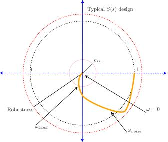
Figure 7. Sensitivity transfer function, S(s), specifications in the Nyquist diagram.
