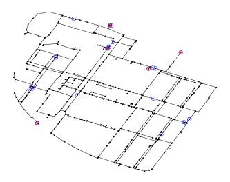
Fig. 4: DMA network sensor placement results under structural analysis approach
