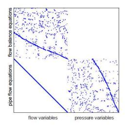
Fig. 2: Structural model of the DMA network
