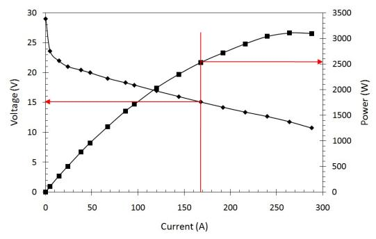
Figure 2. Polarization curve obtained for the 30-cells stack operating under optimal conditions
