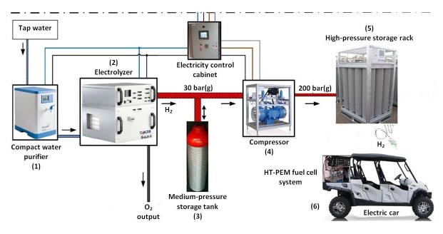
Figure 1. General scheme of the hydrogen production and storage plant together with the end-user commercial electric vehicle properly modified to be powered by a hybrid powertrain
