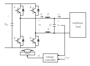
Figure 6. Circuit diagram.
