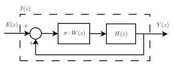
Figure 1. Internal model used in Repetitive Control.
