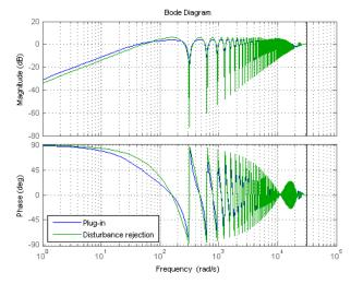
Figure 7. Sensitivity function for RC based on plug-in and disturbances observer approaches.
