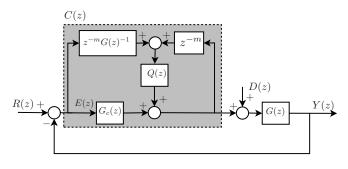
Figure 4. RC : Disturbance rejection approach.
