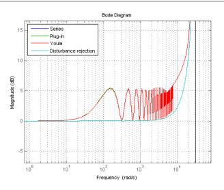
Figure 10. Bode diagram of 1/T(z) for all four approaches.
