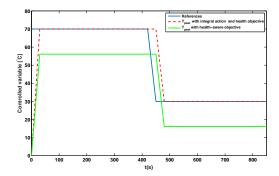
**Figure 8.** Evolution of pasteurization temperature with (red) and without (green) integral action in the MPC.
