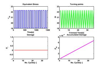
Figure 2. Rainflow counting damage estimation.
