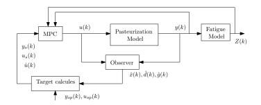
**Figure 7.** Representative block diagram of the predictive control system with linear regulator and fatigue model.
