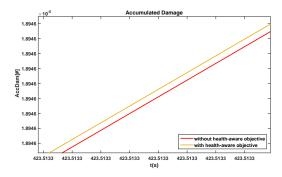
**Figure 9.** Evolution of accumulated damages with (yellow) and without (red) health-aware objective in the MPC.
