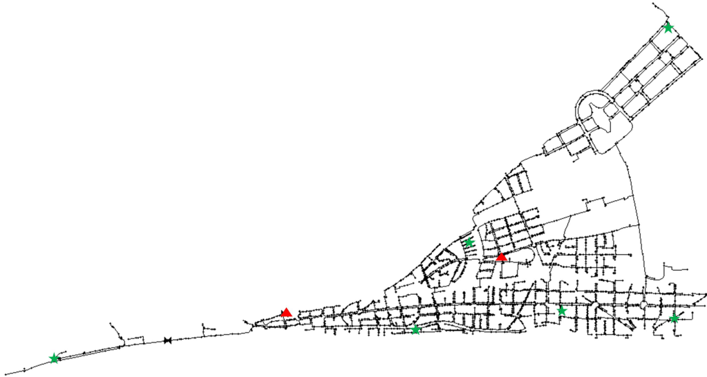
Fig 3 Water network of Castelldefels Platja DMA (EPANET model) highlighting inner pressure sensors (green stars) and DMA inlets (red triangles).
