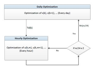
Fig. 4 Upper and Lower layer optimizations of multi-layer MPC
