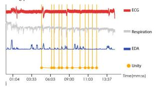
Figure 1: Plot of normalized raw data obtained from different sensors. The bottom part of the graph shows how the signals are aligned with events in the audiovisual content generated by the 3D engine (Unity). The data was collected by sensors and stored in the URDB in real-time during an experiment in XIM.
