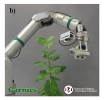
Setups for robot perception and manipulation of deformable objects at IRI: a) perceiving and handling clothes [2, 3, 9, 14], b) measuring the chlorophyll of plant leaves for phenotyping [5, 6].
