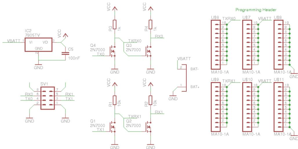
**Figure 2:** MR-C3024 expansion board schematic with 1 k $\Omega$  pullups.
