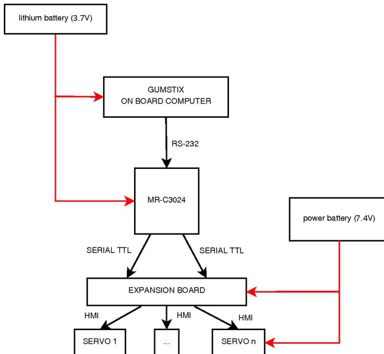
Figure 4: Robot's architecture
