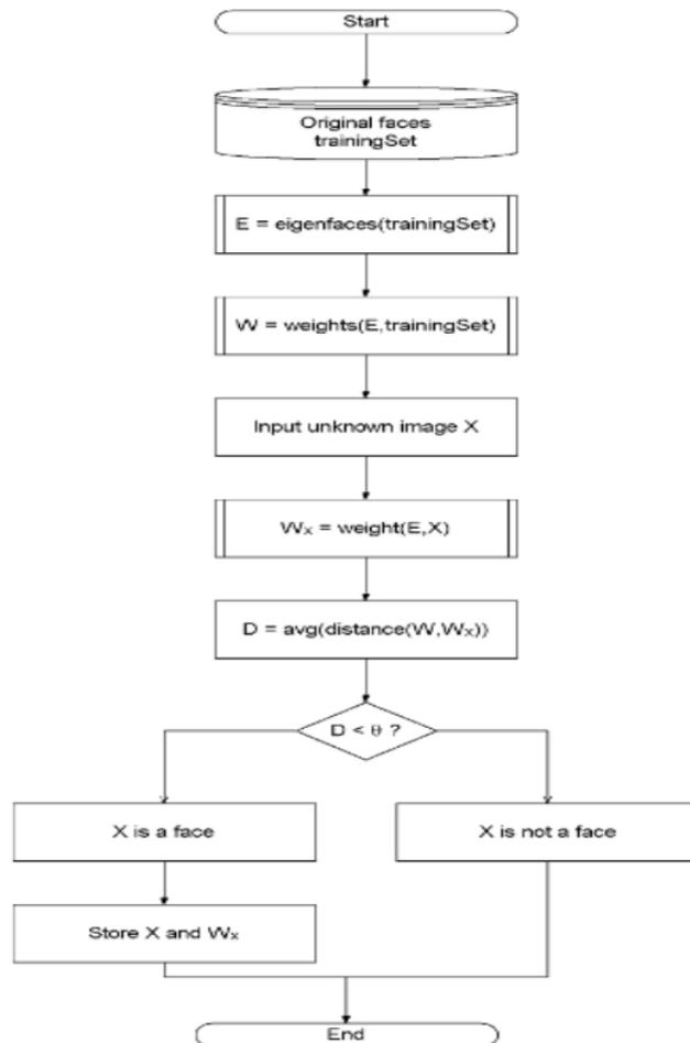
Figure 3.8: The flow of the Eigenface algorithm. Source : [16]
