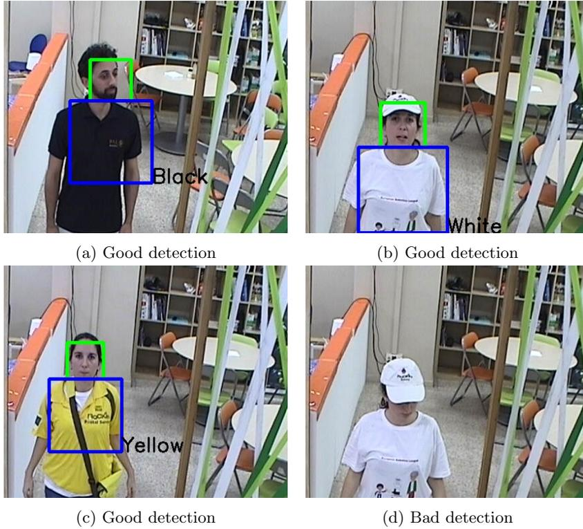
Figure 6.3: Results of face, body and color detection during the ERL competition
