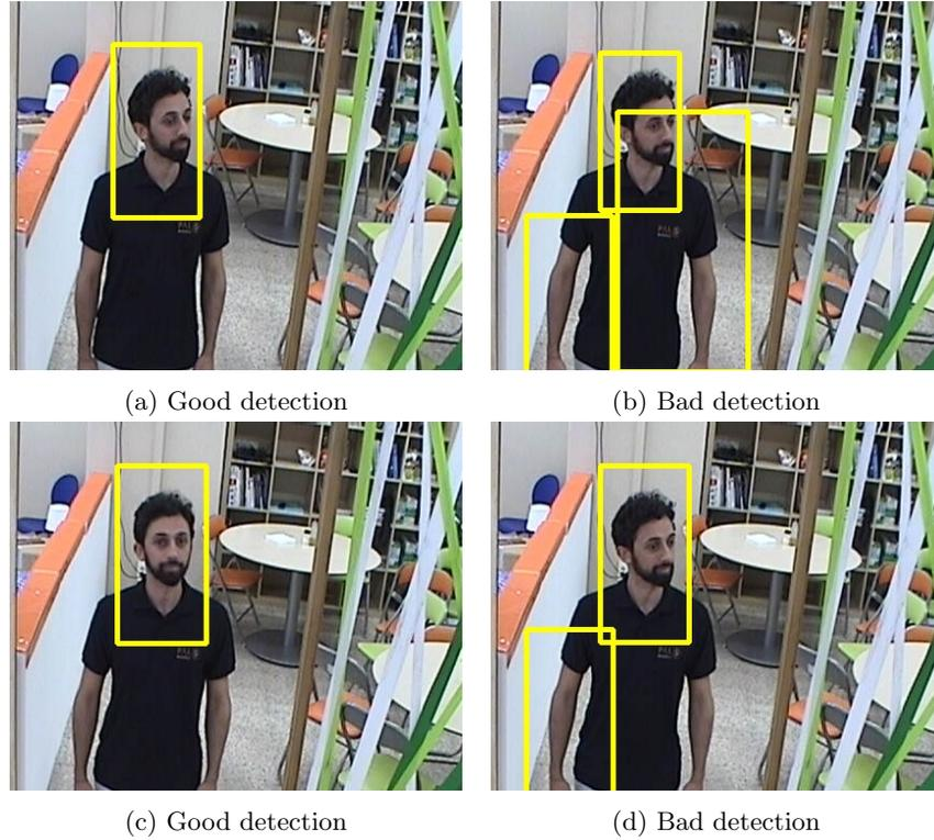
Figure 6.1: Results of HOG for person detection
